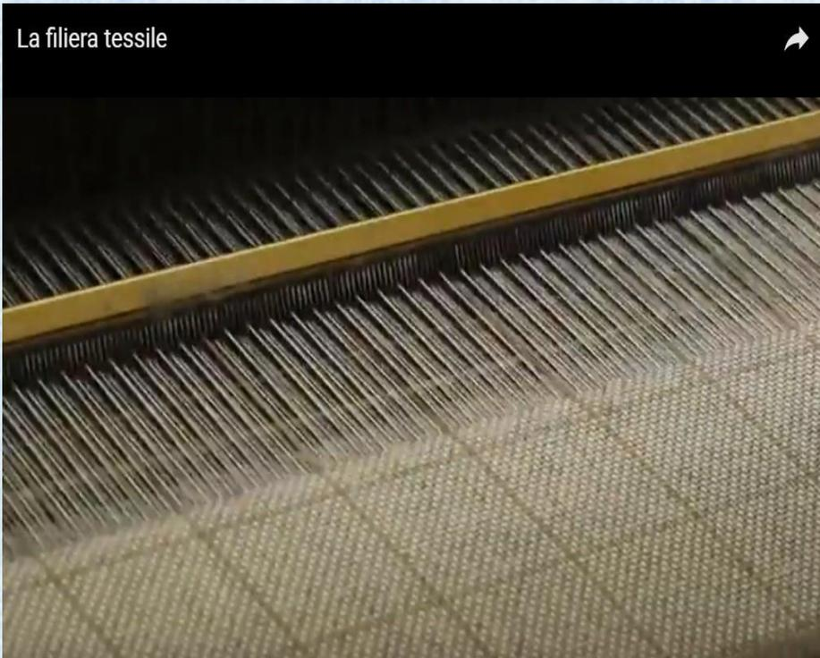
The weaving starts with the warping, that means the production of a parallel bundle of wires according to an order pre-established by the designers. The pre-arranged threads form the warp that will intersect with other wires to make up the plot.
