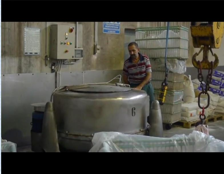
The colors are dosed carefully to get the right shades .Fibers are immersed in water and come pervaded deep from the color,that in a second phase will be stabilized.
